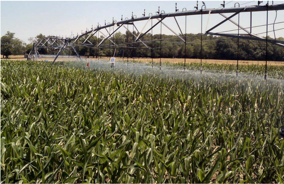
Irrigating corn with one of SIRP's 2-tower center pivot systems. Soil moisture station is visible in the center of the photo.
