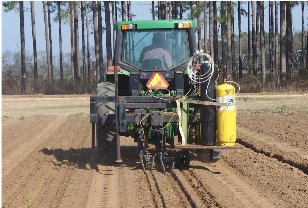
Applying fumigant to vegetable plots.
