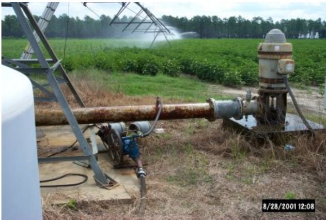
Figure 1. Because wells can be drilled almost anywhere in the high-yielding Floridan Aquifer of Southwest Georgia, the wells are commonly placed at the pivot points.
