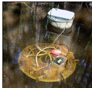
Figure 2. SOD chamber with datalogging computer
