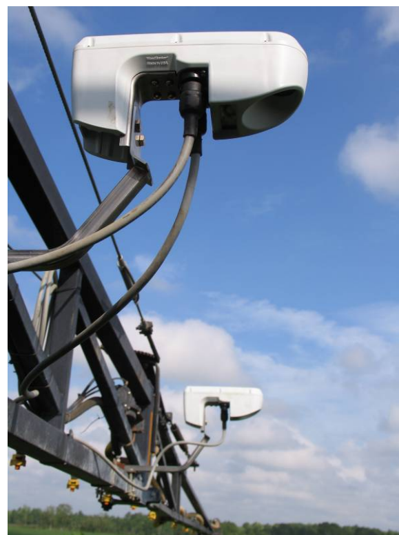
Figure 2. Two of the 6 GreenSeeker ® sensors mounted on the spray boom of the JD6700 high clearance sprayer used in the study.
