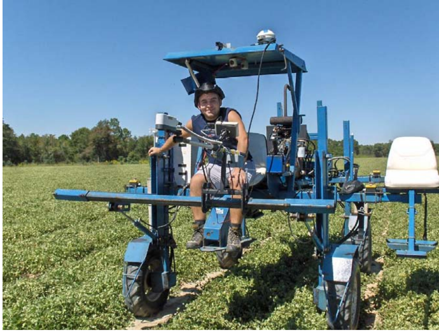
Figure 4. Manuel Renga collects canopy reflectance data using the Crop Circle sensor.
